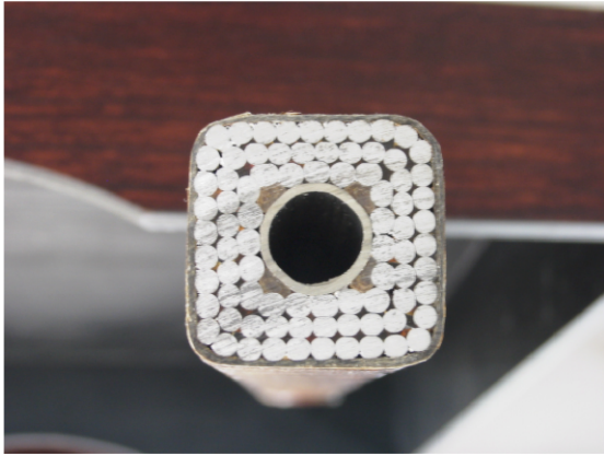
Figure 3: Water-cooled Stranded Conductor Cross-section.
