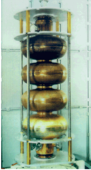
Figure 3. A 4 cell Niobium coated cavity in the clean room.
