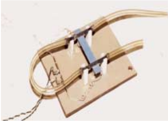
Figure 1: Foto of the SSD heat bridge prepared for studying the temperature distribution along the bridge. Thickness 320 microns, length 70mm. Thermal conductivity 300W/mK. The heat bridge is mounted with two triangular carbon fiber cooling arteries. The heater (representing dummy chips) is glued below the bridge.
