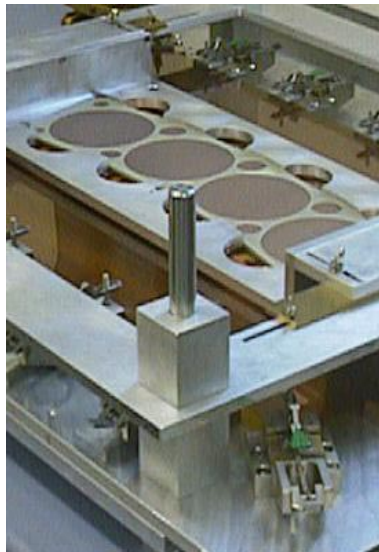
Figure 4: View of the gluing jig. It shows the aligned top frame above the GEM stretched by means of spring-loaded clamps. The aligned spacer frame below the GEM is not visible.
