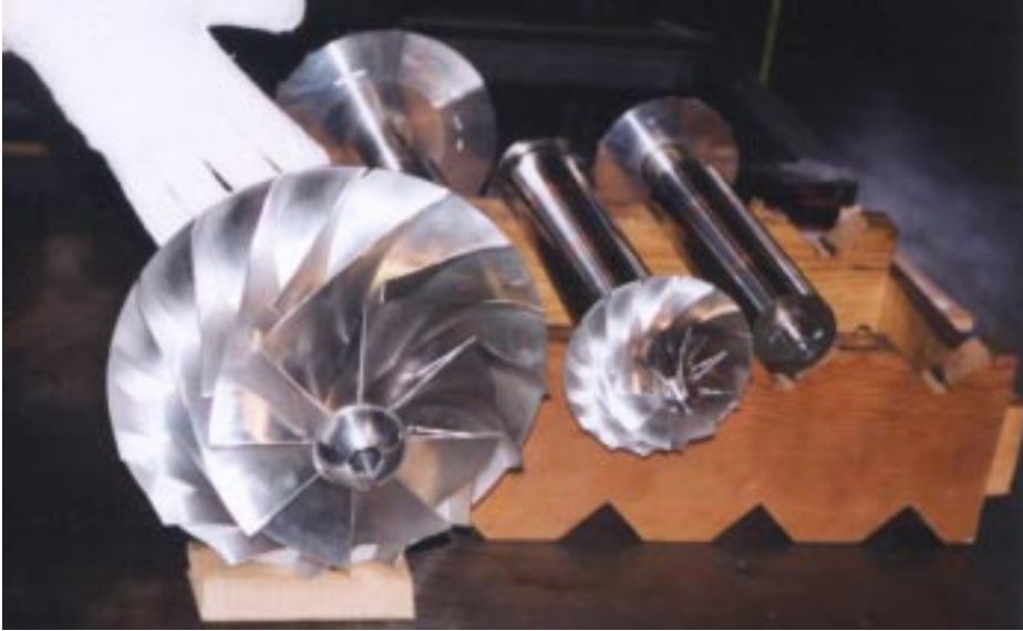
FIGURE 10. Impellers of cold compressors for the first 2.4 kW @ 1.8 K refrigeration unit
