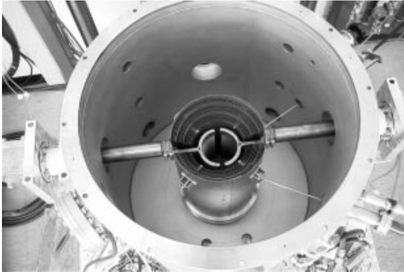
Fig. 3. Photographic view of the furnace, featuring the hot zone with the radiation shield inside the vacuum chamber
