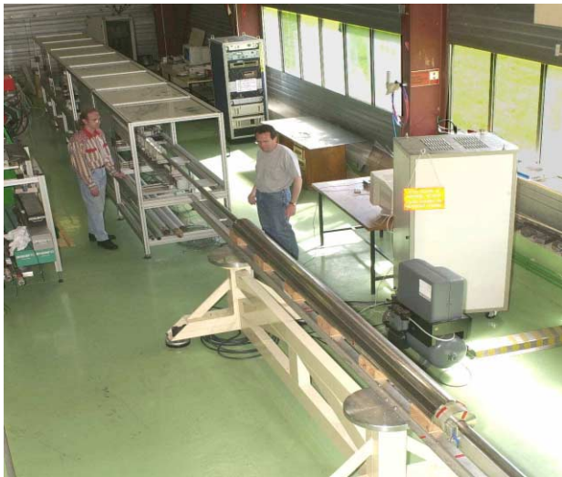
Fig. 1: CEA's station for the warm magnetic measurements with a collared aperture.
