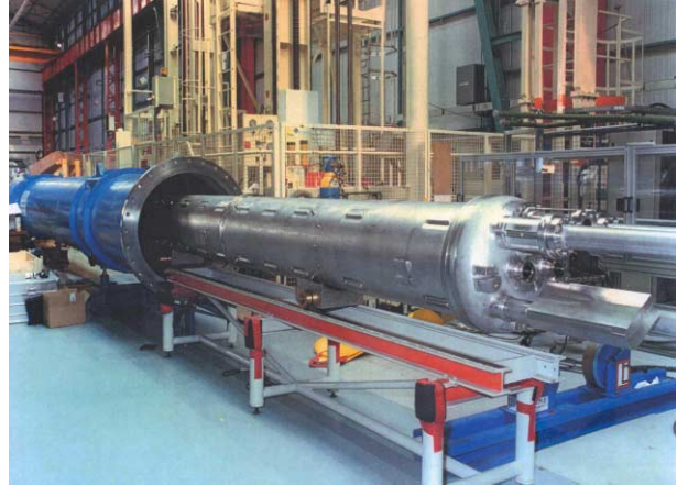
Fig. 2: Insertion of SSS cold mass into the pressure test vessel at CEA-Saclay.
