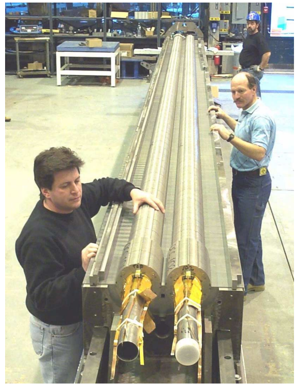
Figure 6: Assembly of the first series D2 separation dipole in BNL.
