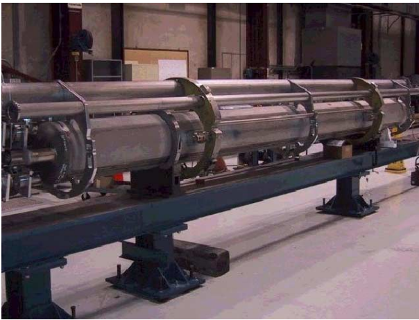
Figure 5: Prototype MQXB low- \beta quadrupole ready for cryostating in Fermilab.
