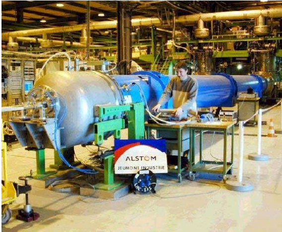
Figure 1: The first pre-series LHC dipole on the test bench in CERN.
