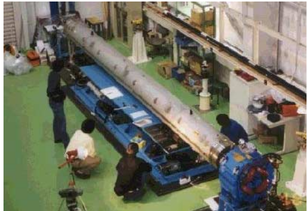
Figure 4: Prototype MQXA low- \beta quadrupole on the warm test bench in KEK.
