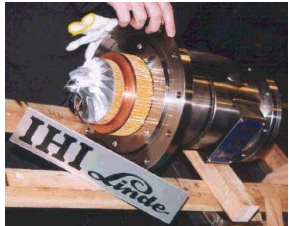
Figure 3: The impeller of the first pre-series cold compressor.
