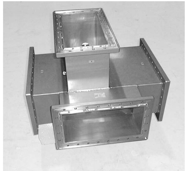
Figure 3: A high-power test model of the asymmetric power divider.
