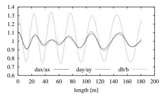
Figure 4: Ratio between the mismatched and matched r.m.s. radii in case of a 30% High-frequency mode excitation for case 1
