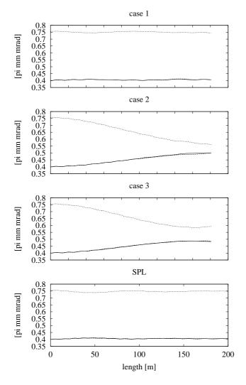
Figure 2: R.m.s. emittance evolution (upper curves: longitudinal, lower curves: transverse)
