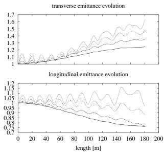
Figure 3: Evolution of fractional normalized emittances for case 2 in ascending order: r.m.s., 99%, 99.9%, and 99.99%
