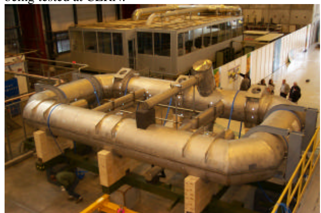
Figure 2: The B_0 toroid magnet test coil at CERN
