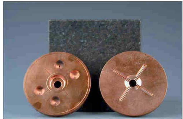
Figure 8: Machining test of 30 GHz slotted iris disks.
