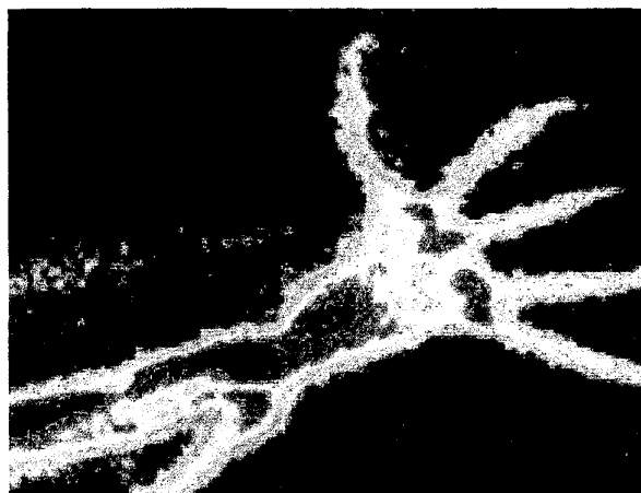
Fig. 14: X-Ray radiography of the foot of a micro-mammal, made with the 2-D GEM detector. The image size is 9x7 \text{mm}^2 .
