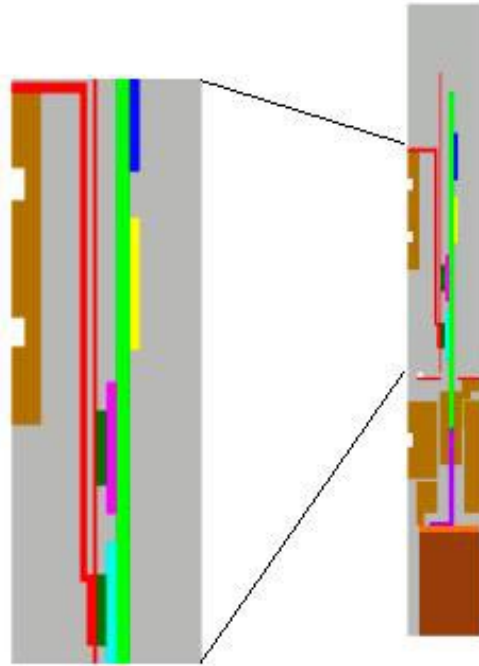
Figure 6 - Case 1: Low connection and no foam at upper chips.
