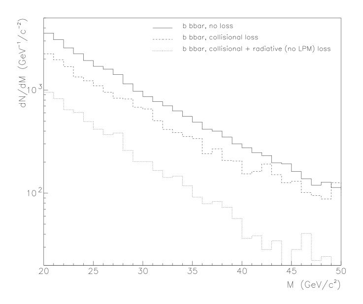
Figure 2: Invariant mass distribution of  $\mu^+\mu^-$  pairs from  $b\overline{b}$  decays with  $p_T^\mu > 5$  GeV/c and  $|\eta^\mu| < 2.4$  for various scenarios: without energy loss (solid histogram), with collisional loss only (dashed histogram), with collisional and radiative loss in incoherent limit (dotted histogram). Nuclear shadowing has been included.
