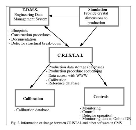
Ultimately, CRISTAL may be required to provide EDMS with some of these physics parameters for future upgrades of the experiment. Hence, CRISTAL is both a client of and a server for data from EDMS and an interface will need to be specified for this sharing of data.
