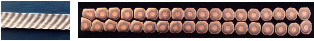
Figure 2.11: The LHC Rutherford cable for the outer layer of the main dipole magnets, quadrupole magnets and busbars: 36 strands, width 15.1 mm, J_c(1.9\text{ K}, 9\text{ tesla}) \geq 12900\text{ A} , A = 19.2442\text{ mm}^2 , strand twist pitch L_p^s \approx 10.5\text{ cm} . A short longitudinal section is shown on the left; the trapezoidal cross-section on the right.
