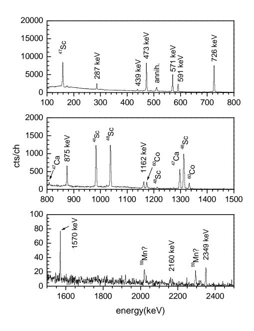
Figure 2:  $\beta$ -delayed  $\gamma$  spectrum observed in the coaxial Ge detector.
