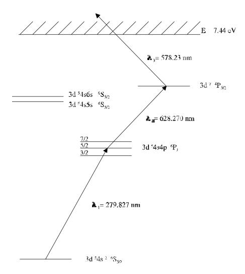
Figure 1: Laser ionization scheme used in this work for Mn.
