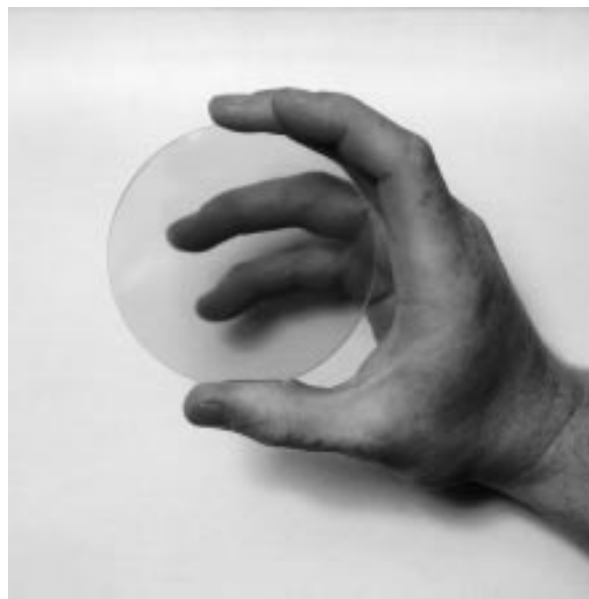
Figure 1: Free-standing, 100 mm diameter CVD diamond (courtesy of De Beers Industrial Diamond Division (UK) Ltd.) [1].
