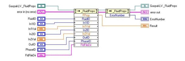
The subVI *GaspakLV FProp.vi* uses the LabVIEW ActiveX *Invoke Node* to call the function *FProp* of the Automation refnum created before. Afterwards a *Property Node* is used to check the result of the internal error handling routine. The subVI can only be used after an instance of the class *FluidProps* has been created in the memory.
