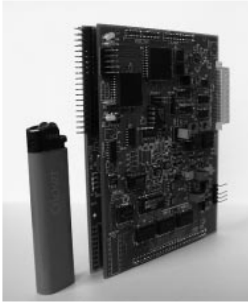
Fig. 7. Photograph of a data acquisition unit for the Compton camera.
