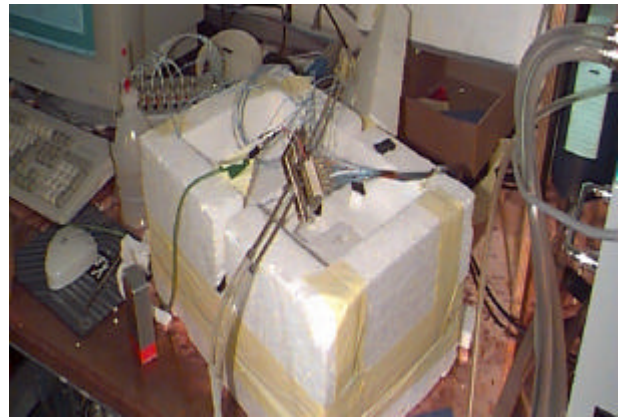
Figure 5: Experimental set-up. Conductive rubber can be seen between electronics boards.
