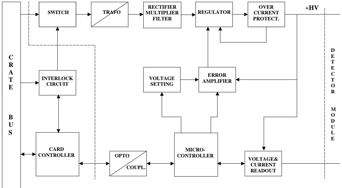
Figure 1. Block diagram of the HV channel
