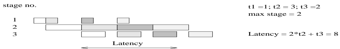
Figure 7.19: Example of latency calculation for a pipeline.
