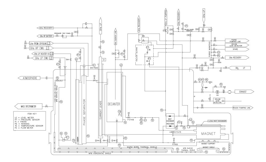
Figure 1 The process flow diagram
