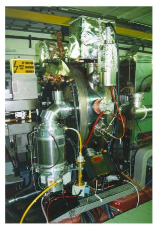
Fig. 46 Installed 80 MHz cavity. The final amplifier can be seen in the foreground.
