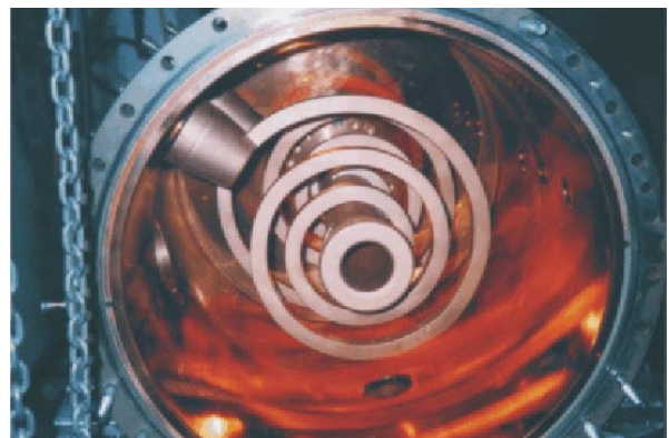
Figure 5: View inside 36 MHz 1.4 MeV/u rebuncher
