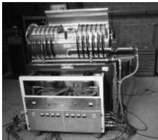
Fig.1 Set-up of the system in the LNS early version, with the 2x50 kW COSY amplifier based on Thomson TH120 tetrodes.
