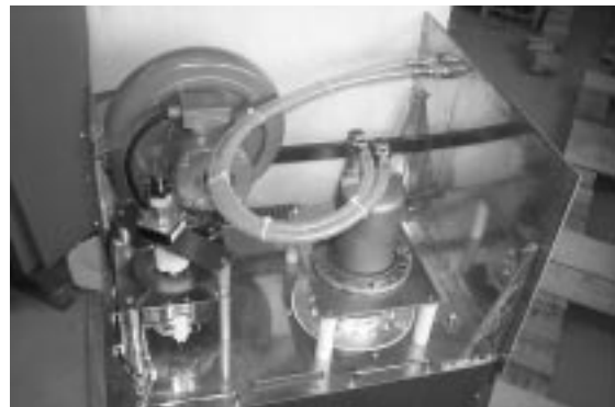
Fig.7 The amplifier module during construction. On the right the RS 1084 power tube mounted on its socket, on the left the motorised VARIAC and an air-cooler fan. Dimensions: width 530, height 690, depth 720 mm.
