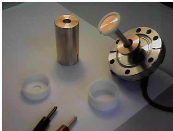
Figure 3-11: pick-up probe (1) and cup (2)
