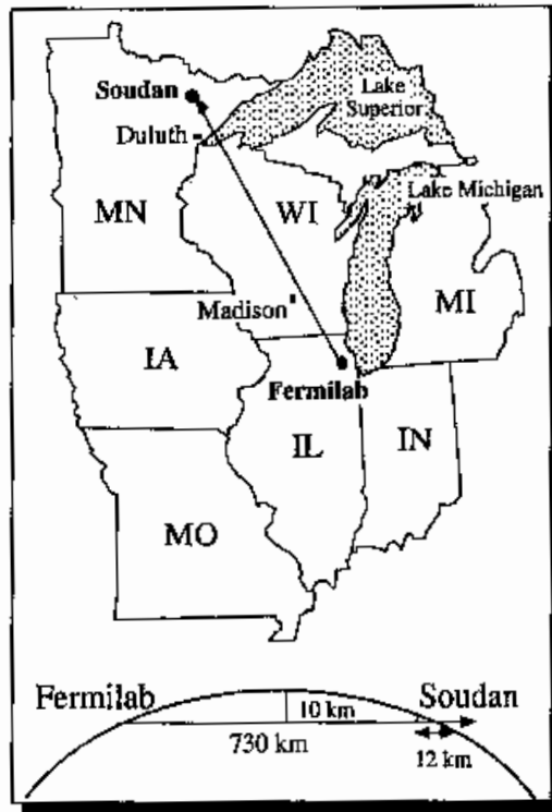
Figure 26: The trajectory of the MINOS neutrino beam from Fermilab to the Soudan mine.
