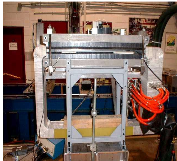
Fig. 1 – Transmission line magnet test stand including 1 meter long laminated steel cores and 100kA-turn copper coil with ten individual water circuits.
