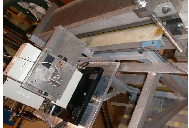
Fig.3 - Stage and Measuring Coil
