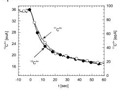
Fig.4 Current decay for a 11C6+ ion beam after extraction from the cyclotron during the first minute of activity release from the cryogenic trap in comparison with the stable 12C4+ ion beam decay.
