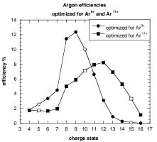
Fig.1 Ionization efficiency distribution for argon spectra optimized on  $Ar^{9+}$  and  $Ar^{11+}$  with oxygen as support gas. The open symbols indicate the mixed ion species.
