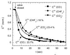
Fig. 3 Normalized current decay for C<sup>4+</sup> ion beams from CO, CO<sub>2</sub> and CHF<sub>3</sub> calibrated leaks with the AECR-U ion source.
