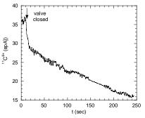
Fig.5 Current decay for a <sup>11</sup>C<sup>6+</sup> ion beam after extraction from the cyclotron after 12 minutes of continuos release from the cryogenic trap
