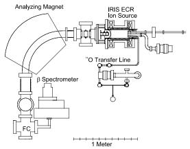
Fig. 6 Schematic of the new exotic ion beam test stand and the <sup>14</sup>O experiment.
