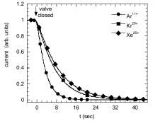
Fig.2 Normalized beam current decay for selected charge states for a few noble gases with the LBNL AECR-U ion source.
