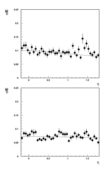
Figure 5: The dependence of the energy resolution on pseudorapidity for charged pions of constant transverse energy:  $E_T=20~{\rm GeV}$  (top plot) and  $E_T=50~{\rm GeV}$  (bottom plot). The lines correspond to the energy resolution parametrised using Equation  $\sigma/E=39\%/\sqrt{E}\oplus 1\%$  for  $E_T=20~{\rm GeV}$  and  $\sigma/E=49\%/\sqrt{E}\oplus 2\%$  for  $E_T=50~{\rm GeV}$ .
