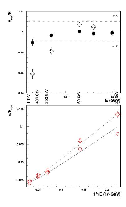
Figure 4: Pion energy scan in the extended barrel ( $\eta=1.3$ ). The top plot shows the residual non-linearity, the bottom plot shows the energy resolution with the results of the fit with Equation  $\sigma/E=a/\sqrt{E}\oplus b$ . Two sets of parameters for the pion energy reconstruction have been used: open crosses — for energy independent parameters; solid dots — for parameters fitted at each energy and pseudorapidity.
