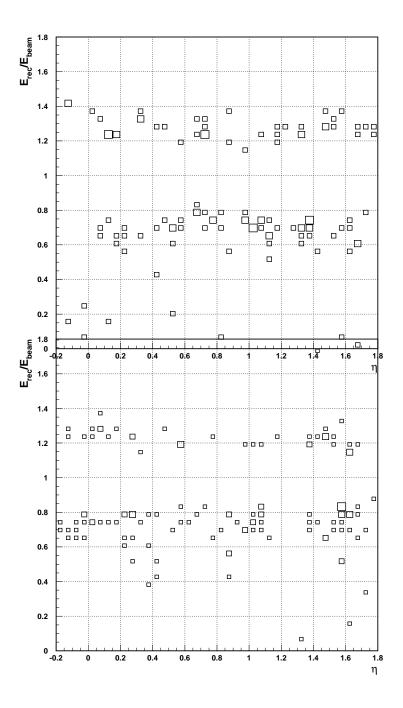
Figure 7: Events in the tails of the distribution of the reconstructed energy as a function of pseudorapidity for pions of  $E_T = 20$  GeV (top plot) and  $E_T = 50$  GeV (bottom plot). Tails are defined as events with reconstructed energies more than three standard deviations away from the mean.
