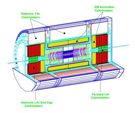
Figure 1: Three-dimensional cutaway view of the ATLAS calorimeters.
