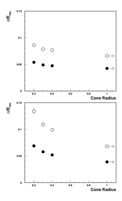
Figure 9: Energy resolution for 50 GeV (open circles) and 200 GeV (solid dots) charged pions at  $\eta=0.3$  (top plot) and  $\eta=1.3$  (bottom plot) as a function of the cone size. The points with the arrows correspond to the case without restriction to a cone. Energy and pseudorapidity dependent parameters were used for the energy reconstruction.
