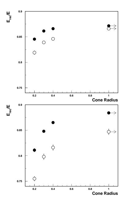
Figure 8: Energy response for 50 GeV (open circles) and 200 GeV (solid dots) charged pions at  $\eta=0.3$  (top plot) and  $\eta=1.3$  (bottom plot) as a function of the cone size. The points with arrows correspond to the case without restriction to a cone. Energy and pseudorapidity independent parameters were used for the energy reconstruction.
