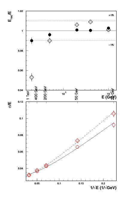
Figure 3: Pion energy scan in the central barrel ( $\eta=0.3$ ). The top plot shows the residual non-linearity, the bottom plot shows the energy resolution with the results of the fit with Equation  $\sigma/E=a/\sqrt{E}\oplus b$ . Two sets of parameters for the pion energy reconstruction have been used: open crosses — for energy independent parameters; solid dots — for parameters fitted at each energy and pseudorapidity.
