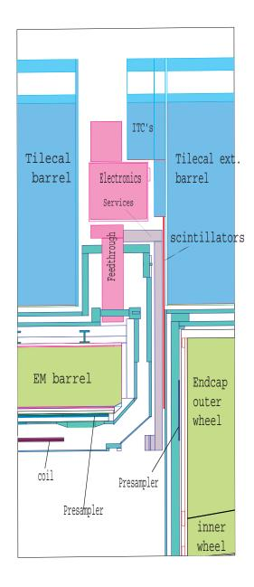
Figure 2: Longitudinal view of a quadrant of the vertical gap between the barrel and extended barrel Hadronic Tile Calorimeter.
