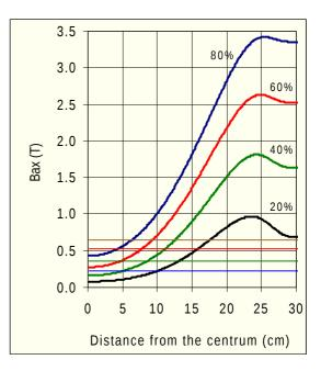
Fig.5. Axial distributions at different coils currents (20-40-60-80%). For symmetrical reasons only half of the curves are drawn.. The horizontal lines represent resonance values for 6.4, 10, 14.5 and 18 GHz.
