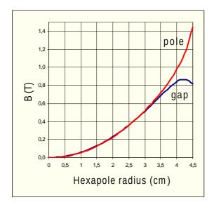
Fig.3. The radial magnetic induction at the poles and the gaps inside the open hexapole
