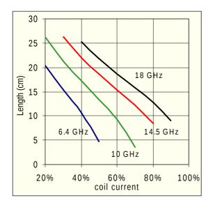
*Fig.7. The length of the resonance zone at different frequencies.*
