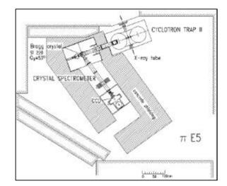
Fig.1. The original cyclotron magnet and beam line arrangement. A very similar arrangement will be used for the proposed experiment.
