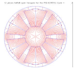
*Fig.2. Cross section view of the open hexapole. ID*=90 *mm, OD*=240 *mm, length*=250 *mm, Br*=1.28 *T, Hcj*=21 *kOe.*
