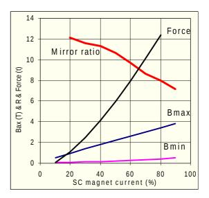
Fig.6. The peak and minimum fields on the axes together with their (mirror) ratio and with the force effects to one of the SC coils.
