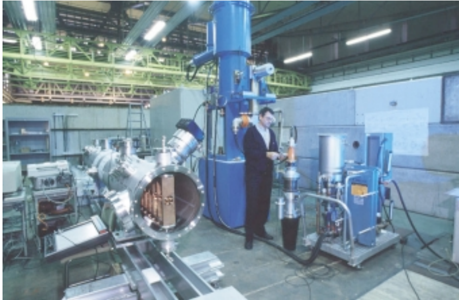
Figure 11: RFQ seen from downstream end, cover removed. In the background the RF amplifier.
