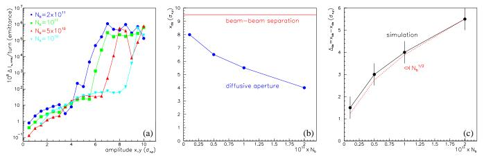
FIG. 14. (Color) Dependence of diffusion due to long-range collisions on the beam current. (a) The change of action variance per turn as a function of the bunch population, (b) approximate diffusive aperture as a function of the bunch population, and (c) same as the left picture, but the vertical axis is the distance to the other beam at the parasitic collision point. A square root dependence is also indicated for comparison.
