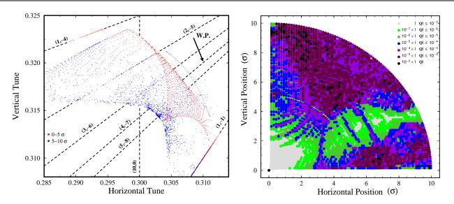
FIG. 3. (Color) Tune footprint and diffusion map for a model including the head-on and long-range collision effect and the KEK triplet nonlinearities, for a 200  $\mu$ rad crossing angle. The symbols are the same as in Figs. 1 and 2.
