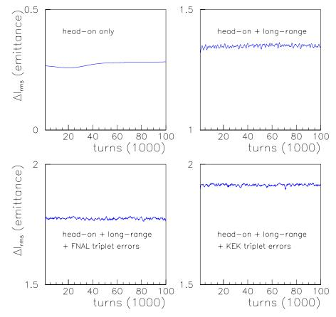
FIG. 6. (Color) The variance in action (in units of rms emittance) for a group of 100 particles as a function of turn number. The particles were launched with identical transverse action corresponding to  $5\sigma_{x,y}$  in both transverse planes and with random betatron phase. The figure demonstrates the effects of head-on collisions, long-range collisions, and triplet nonlinearities, respectively.
