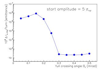
FIG. 15. (Color) The change of action variance per turn as a function of the full crossing angle. The start amplitude is  $5\sigma_{x,y}$  in both planes. The vertical axis gives the variance in units of the design rms emittance times  $10^{-8}$ .
