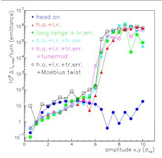
FIG. 8. (Color) The change of action variance per turn as a function of the starting amplitude. Compared are the cases of head-on collisions only, head-on and long-range collisions, long-range collisions plus KEK triplet field errors, both types of collisions plus KEK triplet field errors, the additional effect of a tune modulation at the synchrotron frequency (22 Hz) of amplitude  $10^{-4}$ , and the additional effect of a Möbius twist.
