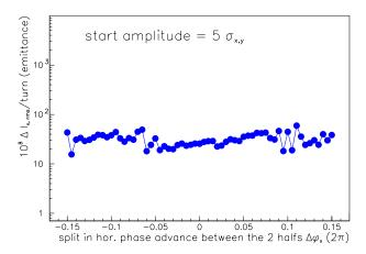
FIG. 12. (Color) The change of action variance per turn (in units of rms emittance times  $10^{-8}$ ) as a function of the difference in horizontal phase advance between the two half arcs. The total horizontal tune is held constant, equal to the nominal. The vertical phase advance per arc is not changed.
