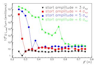
FIG. 17. (Color) The change of action variance per turn as a function of  $\beta_{x,y}^*$ . Along with  $\beta_{x,y}^*$ , the crossing angle is changed, so as to maintain a constant ratio  $\theta_c/\theta_{x,y}$ . The starting amplitude in both planes varies from 3 to  $6\sigma_{x,y}$ . The vertical axis gives the variance in units of the design rms emittance times  $10^{-8}$ .
