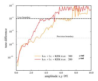
FIG. 16. (Color) The tune variation per 500 turns averaged over the initial x - y amplitude ratio, for two different crossing angles of 300 and 200  $\mu$ rad.
