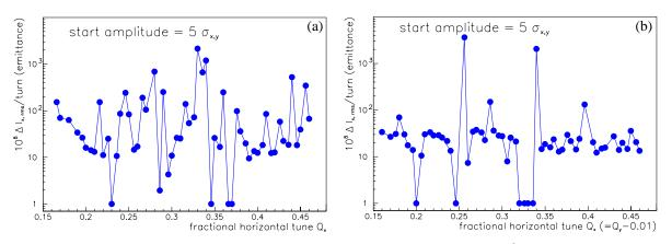
FIG. 11. (Color) The change of action variance per turn (in units of rms emittance times  $10^{-8}$ ) as a function of the horizontal tune (a) for a constant vertical tune and (b) for both the tunes varying so as to keep a constant distance to the (1, -1) coupling resonance. The starting amplitude is  $5\sigma$  in both planes.
