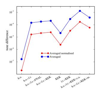
FIG. 5. (Color) Averaged tune differences in logarithmic scale over all particle amplitudes and phases, for different models. The blue curve corresponds to a simple average of the tune change over all tracked particles and the red one to a normalized average by dividing the tune variation of every particle with its initial amplitude.
