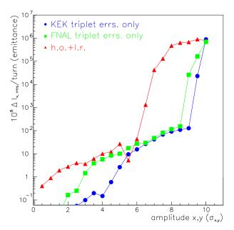
FIG. 9. (Color) The change of action variance per turn as a function of the starting amplitude. Compared are the effect of beam-beam collisions with that of the KEK and FNAL triplet field errors.
