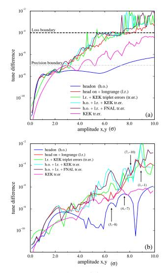
FIG. 10. (Color) The change of frequency per 500 turns (a) averaged over all initial amplitude ratios x - y, and (b) for a fixed initial ratio of 45°, as a function of the starting amplitude. Compared are the cases of head-on collisions only, head-on and long-range collisions, long-range collisions plus KEK triplet field errors, both types of collisions plus KEK triplet field errors, both types of collisions plus FNAL triplet field errors, and only KEK triplet errors.
