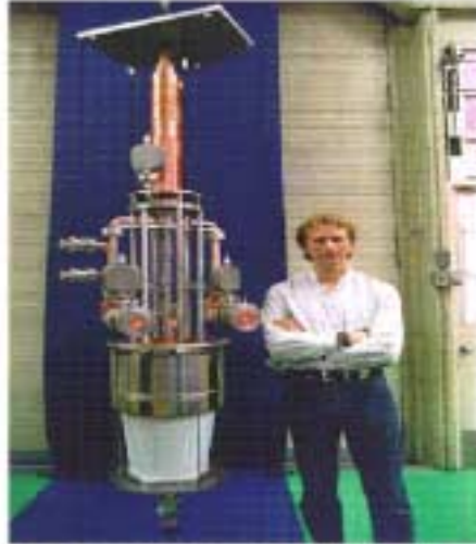
Fig. 16: Photograph of the 50 MW, X-Band, PPM focussed, Klystron developed at SLAC.
