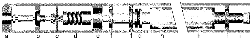
Fig. 2. Schematic drawing of main mole components: (a) multiturn potentiometer, (b) piezo-motor, (c) 3:1 reduction, (d) helical coupling, (e) encoder, (f) ceramic ball bearing, (g) Ti coupling, (h) coil, (i) LED and optics. See text for a detailed description.
