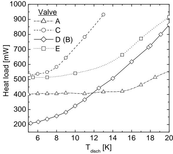
Figure 3. Heat flow to He II vs  $T_{\text{disch}}$
