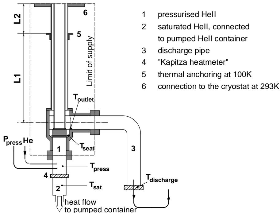
**Figure 2.** Schematic representation of the experimental configuration for the thermal characterisation of the safety relief valves
