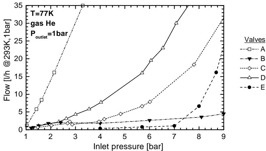
**Figure 1.** Valve leakage at 77K
