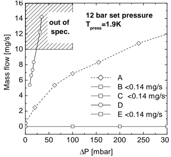
Figure 4. Leakage vs.  $\Delta P$  for 12 bar set mode.
