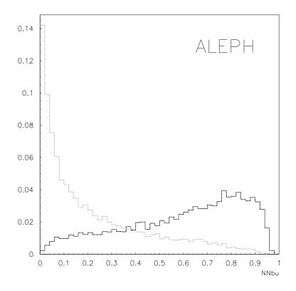
Figure 2: Neural net. output of  $NN_{bu}$  for signal  $b \rightarrow u\ell\nu_{\ell}$  transitions (solid lines) and background  $b \rightarrow c$  transitions (dotted lines). The two Monte Carlo distributions are normalized to the same area.
