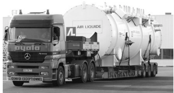
Figure 9: The lower cold box of the first 18 kW cryoplant.
