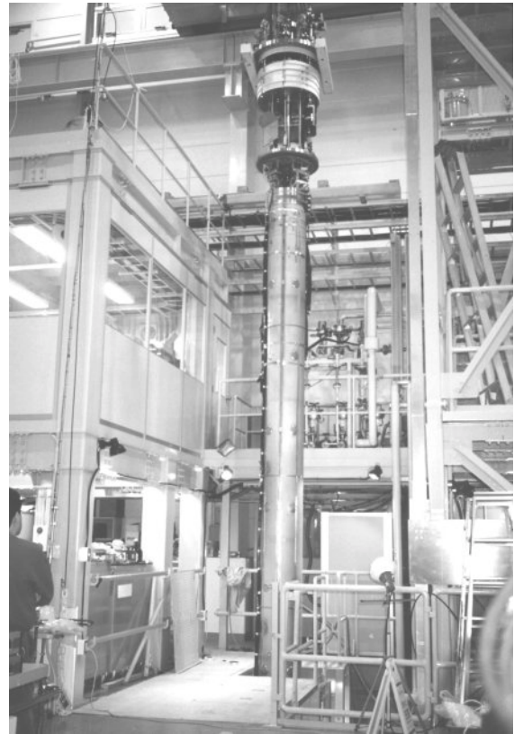
Figure 5: A full-length insertion quadrupole being lowered into a vertical cryostat at KEK.
