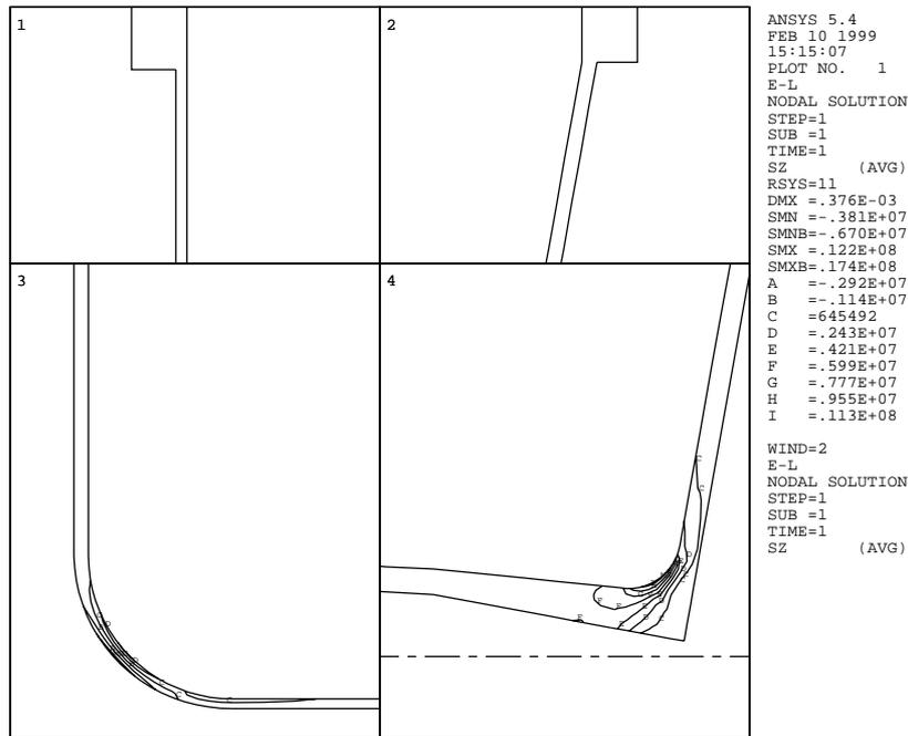
**Fig. 23** Normal stress  $\sigma_z$  (axial) in Pa: typically some 1 to 6 MPa of traction in the tube (not visible on these zoom plots). Bending stress concentration is again nicely visible. Stresses in the end-cap sheet, 'half-way': about C both for entrance and exit.
