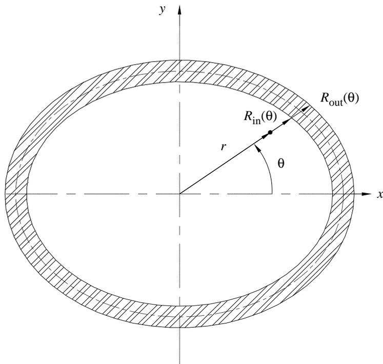
**Fig. 15** Unroundness of inner conductor: geometry definitions.
