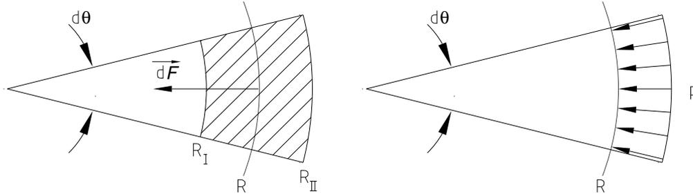
**Fig. 4** Our definition of magnetic pressure  $p$ .
