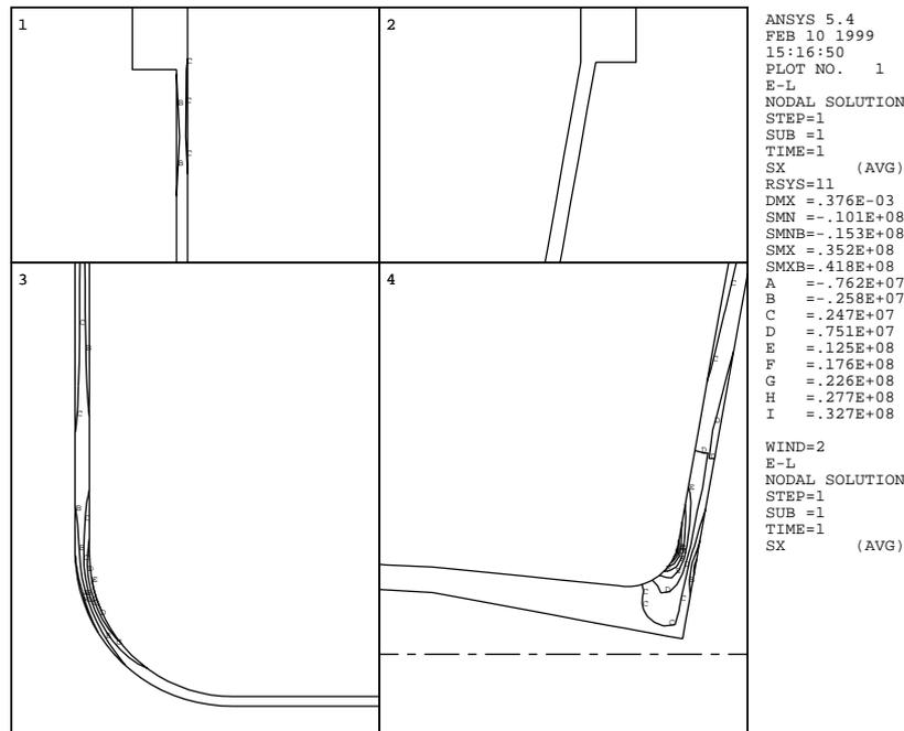
**Fig. 21** Normal stress  $\sigma_r$  (radial) in Pa, positive for tensile and negative for compressive — the usual convention for normal stresses. The diaphragm bending of the end-cap sheet gives a clear concentration effect near the transition. Stress levels in the end-cap sheet, ‘half-way’ between tube and flange (radii 100–200 mm): C to A (from left to right, through thickness) for entrance, about C for exit.
