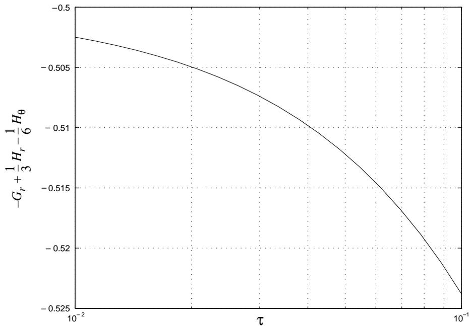
**Fig. 34** A mysterious factor, occurring in bending moment and deflection expressions, mildly varying with thickness ratio. One should keep in mind that the theory loses its validity for higher  $\tau$ .
