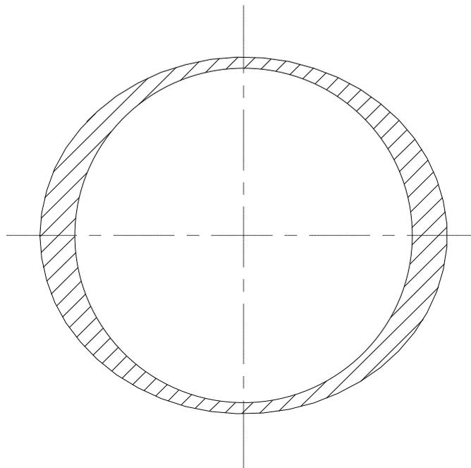
**Fig. 13** Thickness perturbation of  $\cos 2\theta$  type.
