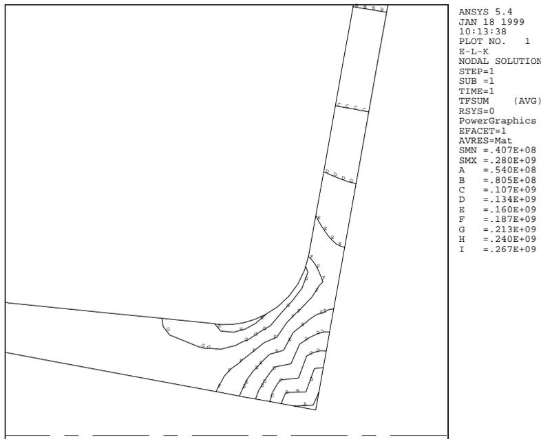
**Fig. 17** Isolines of current density vector magnitudes, in  $\text{A/m}^2$ ; result of the ‘first task’. Unrealistic kinks in the corner region are due to finite element approximation problems, amplified by a distorted grid. The SMN and SMX entries in the legend column are the minimum and maximum values, respectively.
