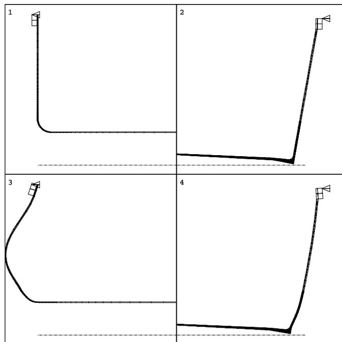
**Fig. 20** Deformations of the horn’s entrance and exit regions: result of the ‘third task’. Top: undeformed. Bottom: deformed, exaggeration factor of 200 applied to deflections. The triangles indicate the boundary conditions: simple axial support. Maximum deflection: about 0.38 mm.
