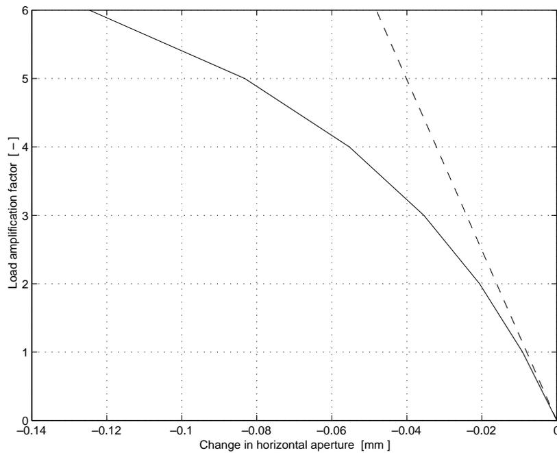
**Fig. 35** Elastic deformations: change in x aperture for a scaled load system ( $\epsilon = 0.1$  mm). Dashed: analytical, only bending effects. Solid: finite element, bending and compression, nonlinear.
