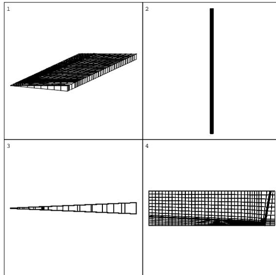
**Fig. 18** Finite element model for the ‘second task’, seen from various viewpoints. For the horn itself, there are eight element layers ‘through-thickness’. The total model contains 995 3D elements, mostly bricks, plus a few wedges. Applied boundary conditions:  $A_r = 0$  at inner radius and at  $z$  end-planes;  $A_\theta = 0$  at  $\theta$  end-planes;  $A_z = 0$  at outer radius.
