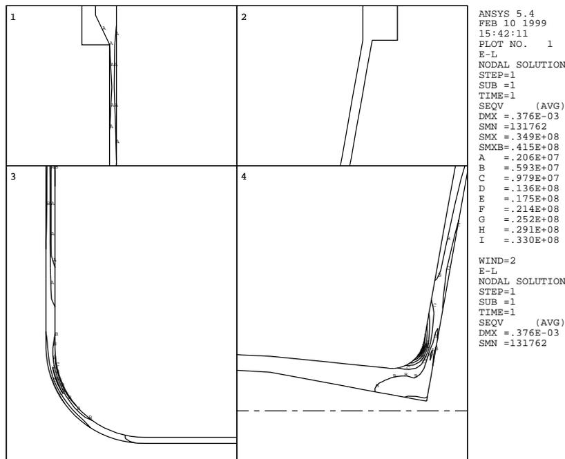
**Fig. 26** Von Mises equivalent stress  $\sigma_{VM}$  in Pa.
