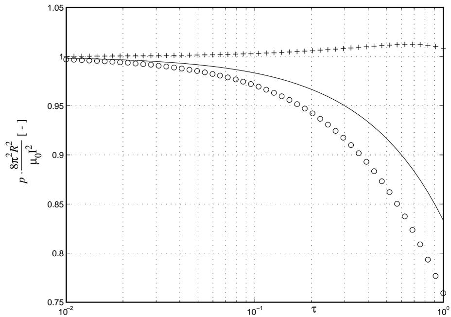
**Fig. 5** Correction factor to the magnetic pressure — expressed in terms of total current  $I$  — as a function of the tube's thickness ratio. Solid line: constant  $J$ . Dots: linearly increasing  $J(r)$ , starting from zero value at  $R_I$ . Crosses: linearly decreasing  $J(r)$ , reaching zero at  $R_{II}$ .
