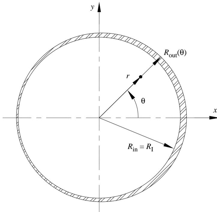
**Fig. 11** Thickness variation of inner conductor: geometry definitions.
