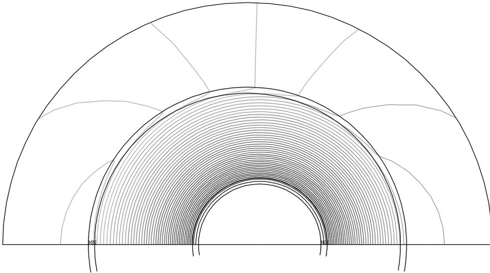
**Fig. 10** Flux lines for a misaligned configuration with arbitrary dimensions, from a finite element test run (lower half not shown for symmetry reasons). The tubes and the model's boundary are also drawn. Only a small portion of 'outer space' seems to have been modelled. In fact, additional elements, mapping towards the infinite boundary, have been deployed.
