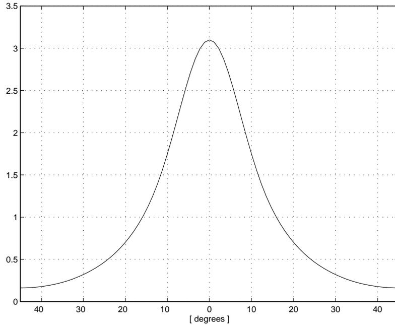
**Fig. 29** Resulting current density (magnitude of vector), 'measured' at station B, as a function of  $\theta$ . Normalized to its average value, being 18.3 A/mm<sup>2</sup>.
