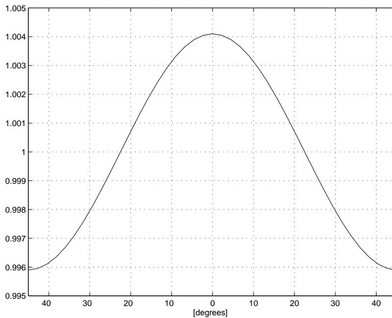
**Fig. 30** Resulting current density (magnitude of vector), 'measured' at station C, as a function of  $\theta$ . Normalized to its average value, being 110 A/mm<sup>2</sup>. Remark: the  $\theta$ -dependence decreases very rapidly as the measurement location is moved downstream.
