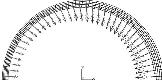
**Fig. 31** Forces on a configuration with arbitrary dimensions and an exaggerated thickness variation, obtained with a finite-element test run.
