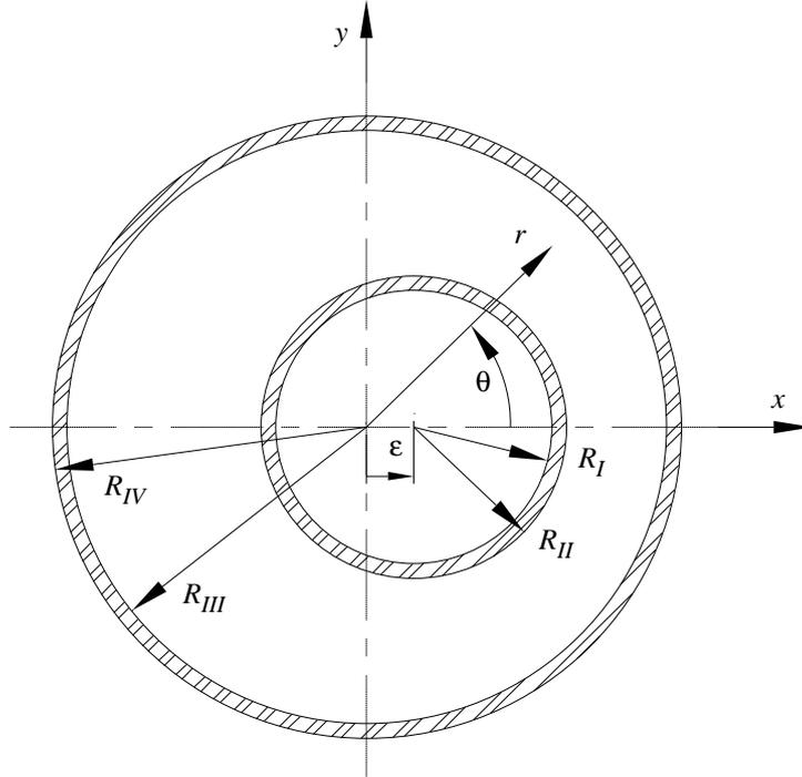
**Fig. 9** Misalignment in  $x$  of the inner conductor: geometry definitions.
