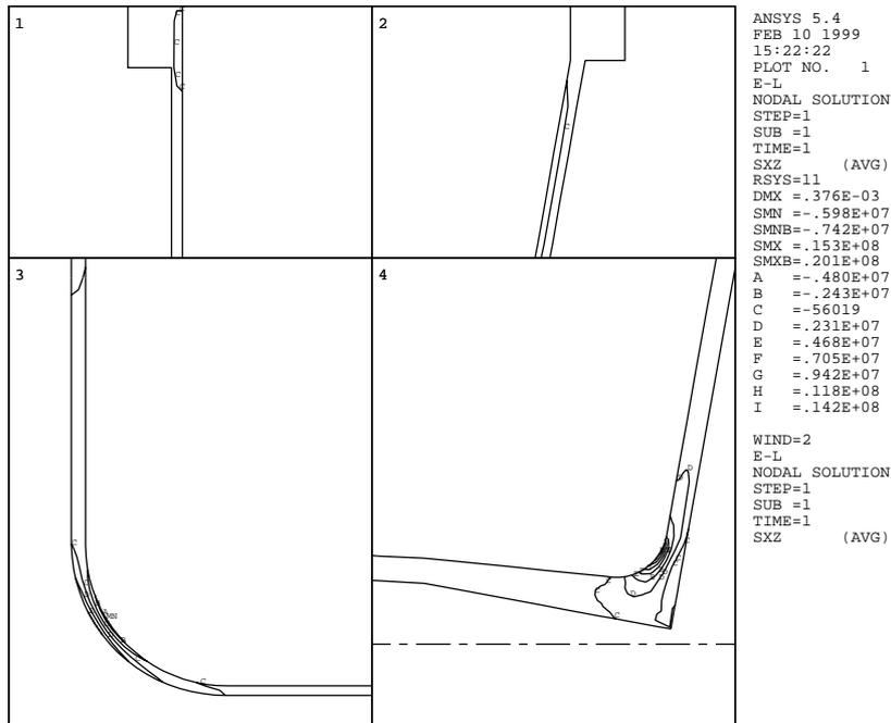
**Fig. 24** Shear stress  $\tau_{rz}$  in Pa. Apart from the ever-present bending effect, there is nothing significant to report. The remaining shear stresses,  $\tau_{r\theta}$  and  $\tau_{\theta z}$ , are zero thanks to axisymmetry. Stresses in the end-cap sheet, ‘half-way’: about C for both entrance and exit.
