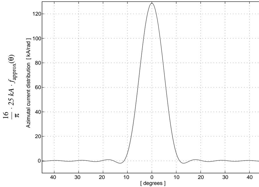
**Fig. 28** Modelled current distribution, injected at station A, as a function of  $\theta$ . The total current for the represented 90-degree arc indeed amounts to 25 kA (curve integration with  $\theta$  expressed in radians).
