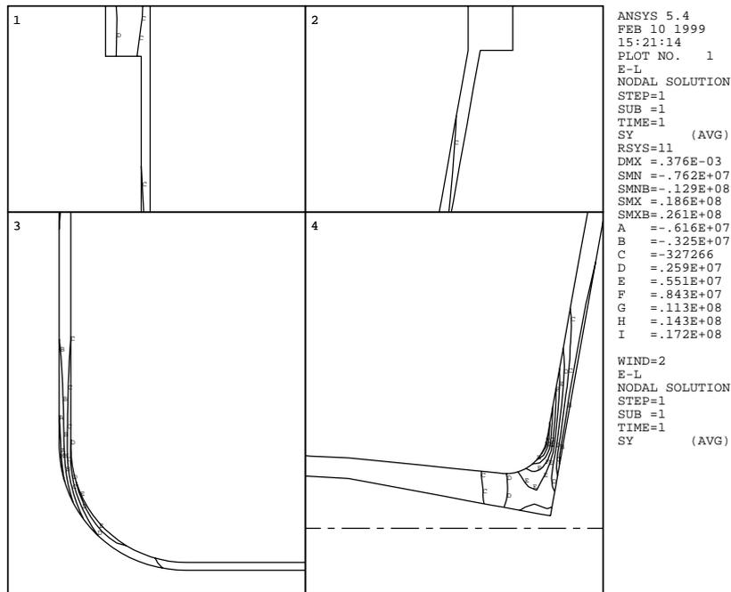
**Fig. 22** Normal stress  $\sigma_{\theta}$  (hoop) in Pa. Horn's tube compression is hardly visible thanks to adequate thickness. End-cap bending is nicely visible. Stresses in the end-cap sheet, 'half-way': C to B for entrance, between B and C for exit.
