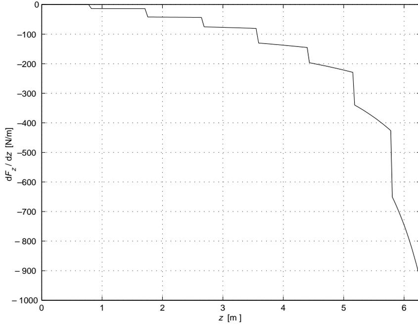
**Fig. 7** Axial force per unit length, resulting from magnetic pressure decomposition. Values are for the first eight portions, cumulating to a  $F_z = -1010$  N. This force will be a part of the loading input for the mechanical finite element model, dealt with in Section 3.
