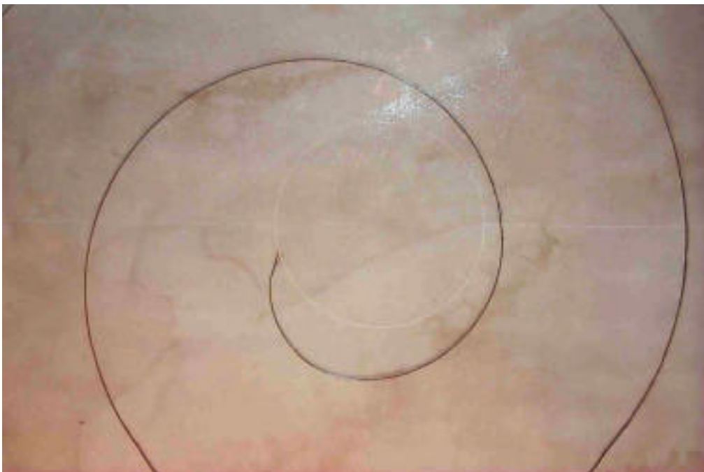
Fig. 4: The kapton spiral used as spacer in the one-mm gaps, glued to an electrode.
