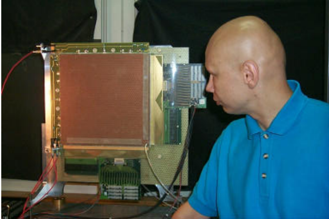
Fig. 5: A fully assembled COMPASS prototype. 128 strips on each coordinate are equipped with readout electronics, but the whole 31 \times 31 \text{ cm}^2 area is active.
