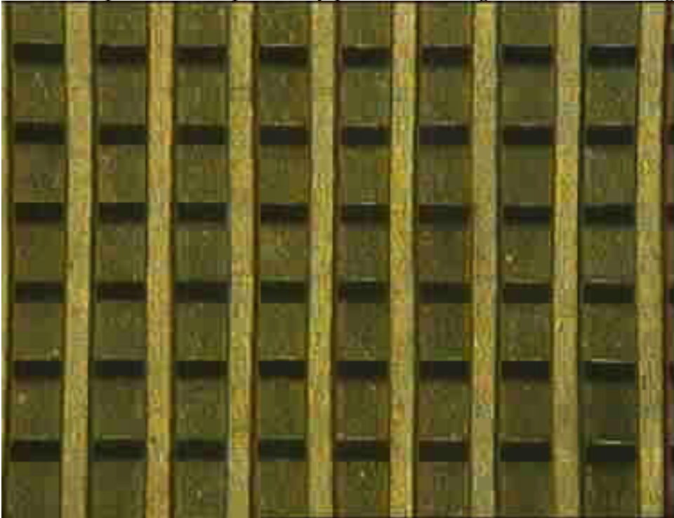
Fig. 3: Close view of the read-out board, with two perpendicular sets of strips, separated by 50 \mu\text{m} kapton ridges. The pitch is 400 \mu\text{m} .
