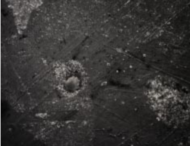
Figure 2: An optical microscope picture (500x) of the back side of the 1.4 mm thick copper iris sample following a single hit by a 10^{10} , \sigma_{x,y} = 15\mu\text{m} round beam, \Delta T \sim 1000 °C. A small melted spot, about 10\mu\text{m} wide, is easily seen.
