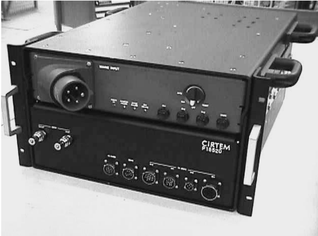
Figure 5: [\pm 600A, \pm 12V] power converter; 6U module.
