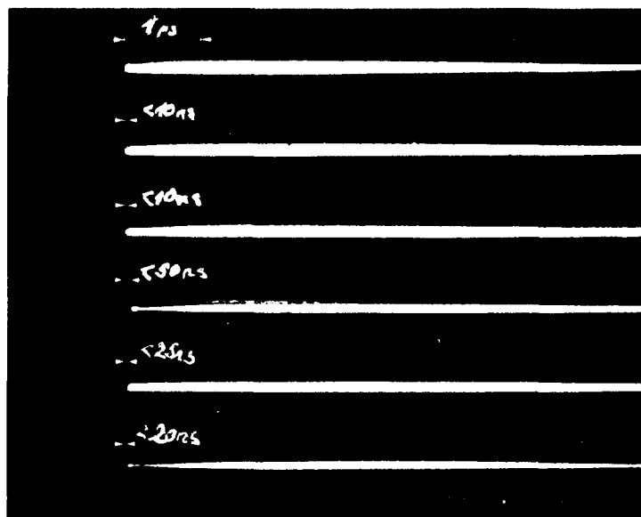
Figure 13b : A typical shadow photograph of the discharges of 6 secondary spark gaps in the configuration drawn in figure 12, using open switches. The initiating circuit is shown in figure 3b, and U_i = 30 kV, K_s = 2,1 .
