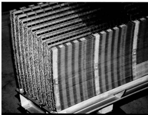
Figure 45: Picture of accordion prototype during its construction.
