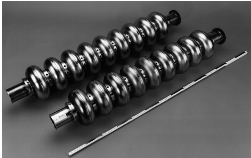
Fig. 2 Nine-cell 1.3-GHz cavities for TESLA. The rounded shape of a typical superconducting cavity design is chosen to suppress multipacting.
