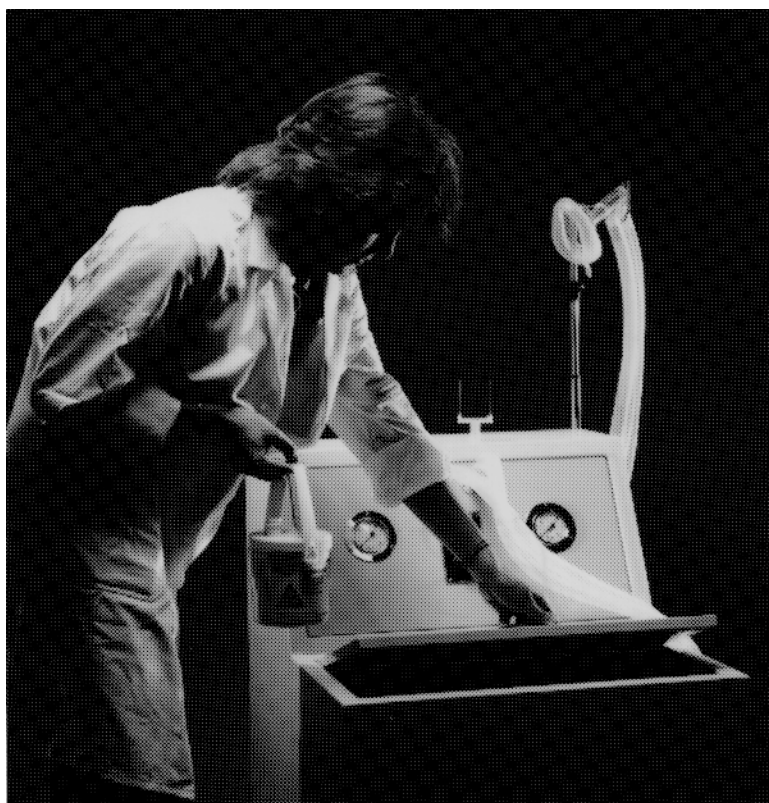
Fig. 12 Rubidium-81/Krypton-81 m generator and Kryptovent II for ventilation diagnostic
