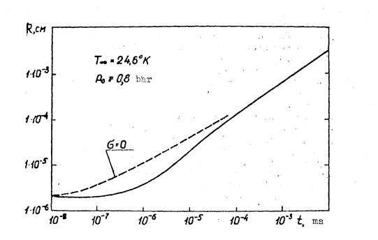
Fig. 4 The dependencies of the embryonic bubble radius upon time: the solid line takes into account surface tension; the dashed line does not consider surface tension ( $\sigma = 0$ ).
