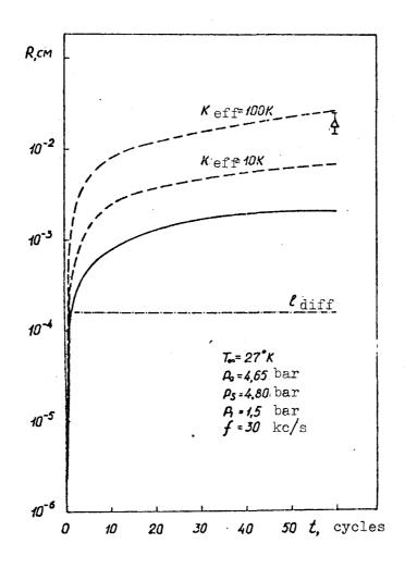
Fig. 1 The dependence of the mean bubble radius upon time in an ultrasonic bubble chamber filled with liquid hydrogen.
