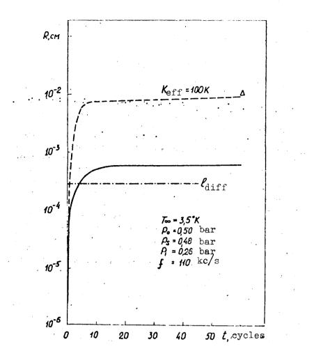
Fig. 2 The dependence of the mean bubble radius upon time in an ultrasonic bubble chamber filled with liquid helium.
