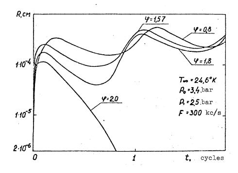
Fig. 3 The dependence of the radius of the embryonic bubble upon time during different phases of the ultrasonic field.
